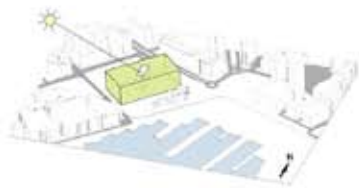
3. A large open space is placed between the four volumes of the museum. The north-south orientation of this void is optimal for the energetic behaviour of the building.
