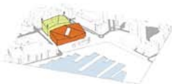
6. The roof of the offices are shaped in such a way that the building is never higher than the museum complex.
