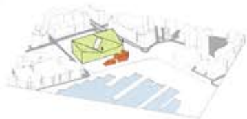
5. The roofline of the museum is lowered to fit the scale of the station buildings.
